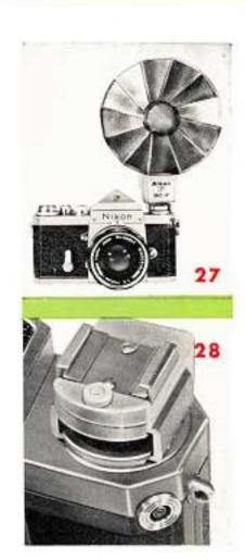
When using FP, M or MF class bulb, select the color of the dot that matches the colored numbers on the shutter speed dial.
