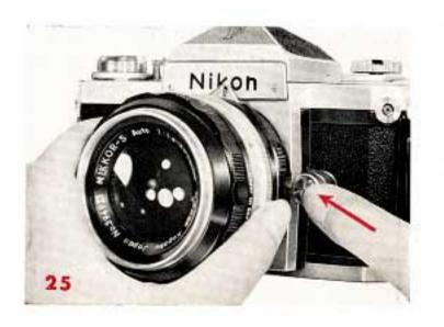
To remove the lens, hold the camera as shown in Fig. 25; depress the lock button and turn the lens barrel clockwise until the black dot on the aperture indicator of the milled ring of the lens lines up with the black dot on the camera body. To mount a lens\*, lining up the black dot on the lens with the black dot on the camera body, press in gently and turn the lens counterclockwise until the lens clicks into position.
