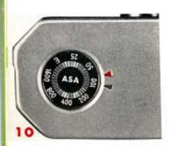
The Film-Speed Reminder Dial (Fig. 10) on the bottom of the camera serves as a reminder of the speed of film (ASA), with which the camera is loaded. It can be set for either color or black and-white film "E" represents "Empty" and may be used to indicate that the camera is not loaded.
