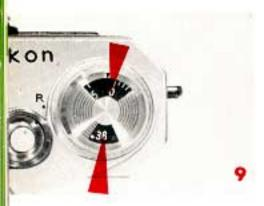
The Exposure Counter (Fig. 9) on the camera automatically returns to one or two spaces before zero when the camera back is removed. After loading the camera, shoot two or three "blank" shots, until the counter registers 1. The camera is now ready for the first shot. Thereafter, the counter will automatically advance consecutively up to 36
