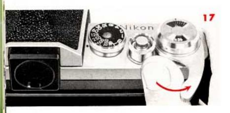
With a single stroke of the advance lever (Fig. 17), the film is advanced, the shutter is wound, and the film counter operates
